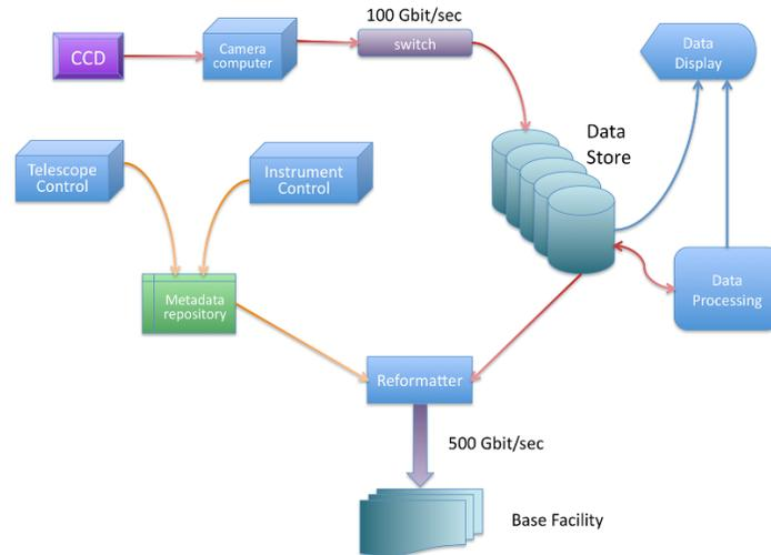
Figure 3. Block-diagram of the reference design for the on-site Data Handling Control System. Details are given in Sect. 3.2.
