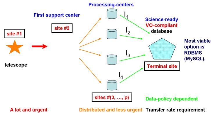
Figure 4. View of the data stream from the telescope to the base center (raw data archive), one or more processing centers ( $I_n$ ), and the terminal VO-compliant database. Details are given in Sect. 3.2.
