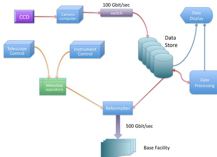
Figure 3. Block-diagram of the reference design for the on-site Data Handling Control System. Details are given in Sect. 3.2.
