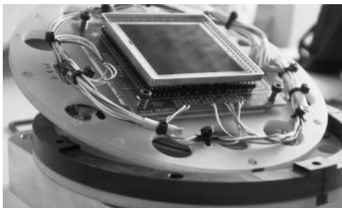
Fig. 3. The SITE CCD mounted on its cold finger before being placed inside the dewar
