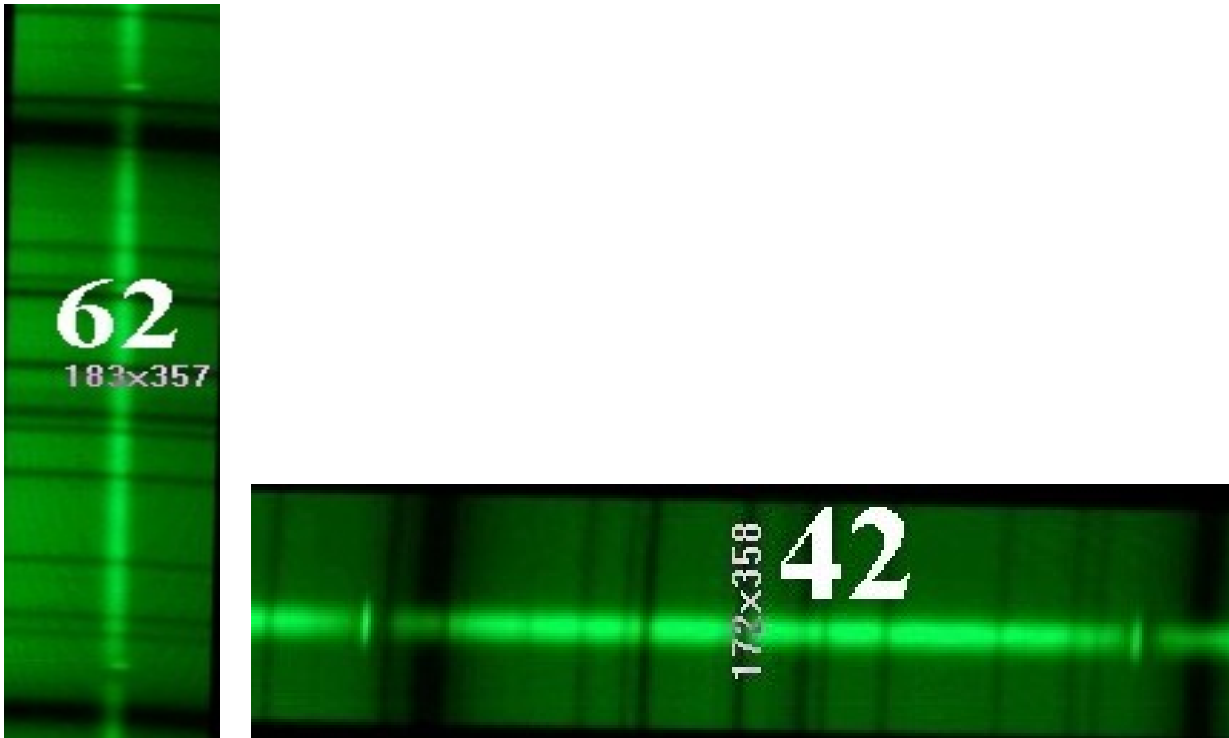
Fig. 3 – Examples of raw spectra obtained with the slit in PA 90° (slit E-W) and PA = 0° (slit N-S) respectively. The long slit permits an accurate subtraction of the night sky continuum. The disk of the planet is spatially resolved, with a seeing PSG varying from 1".2 to 1".8.
