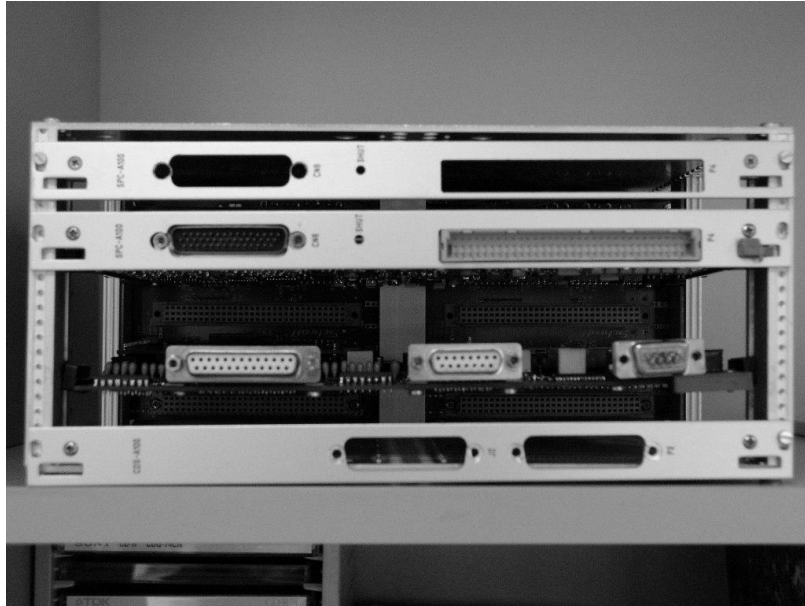
Figure 4. A picture of the new CCD controller, the analog and digital boards can be seen.
