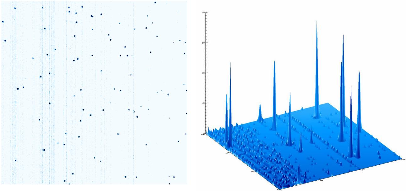
**Figure 9.** Image acquired at 20 MHz clock (160 frames/s) showing several photon events (spots) and 3D plot of a sub area.
