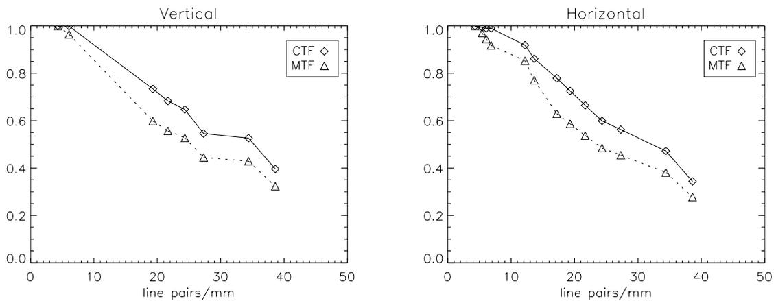
Figure 8. Contrast Transfer Function and Modulation Transfer Function for both directions.
