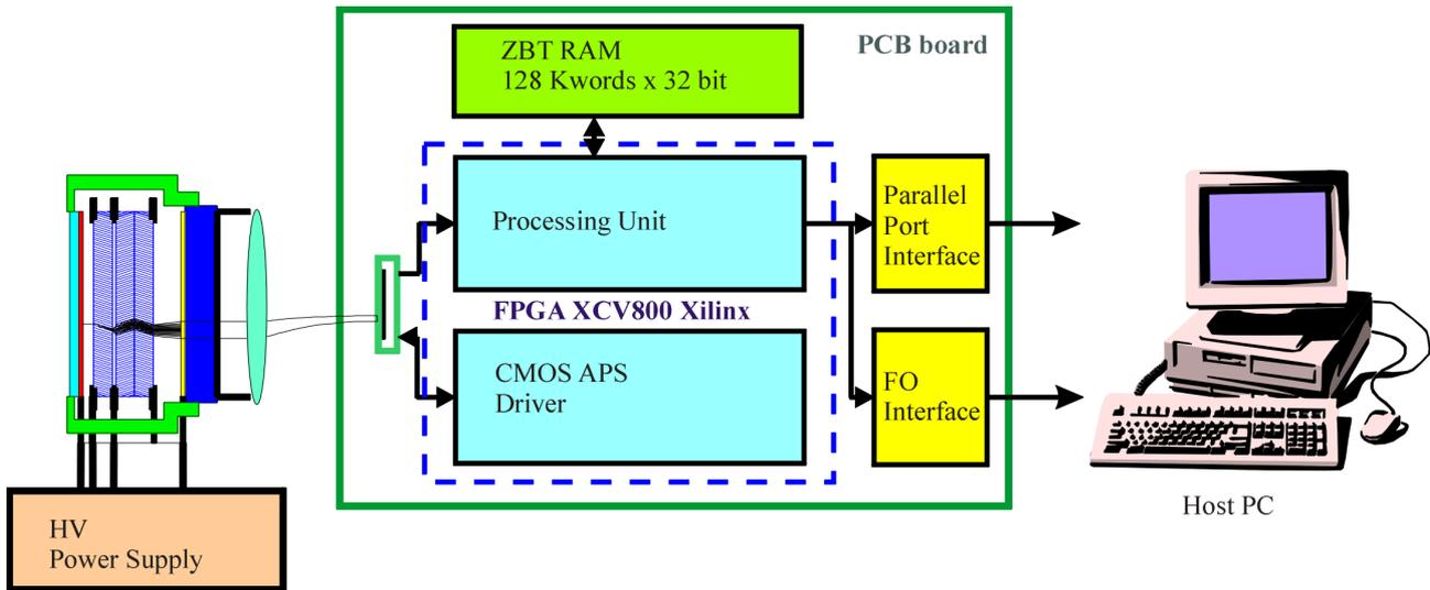
**Figure 1.** Block Diagram of the PC-IAPS.
