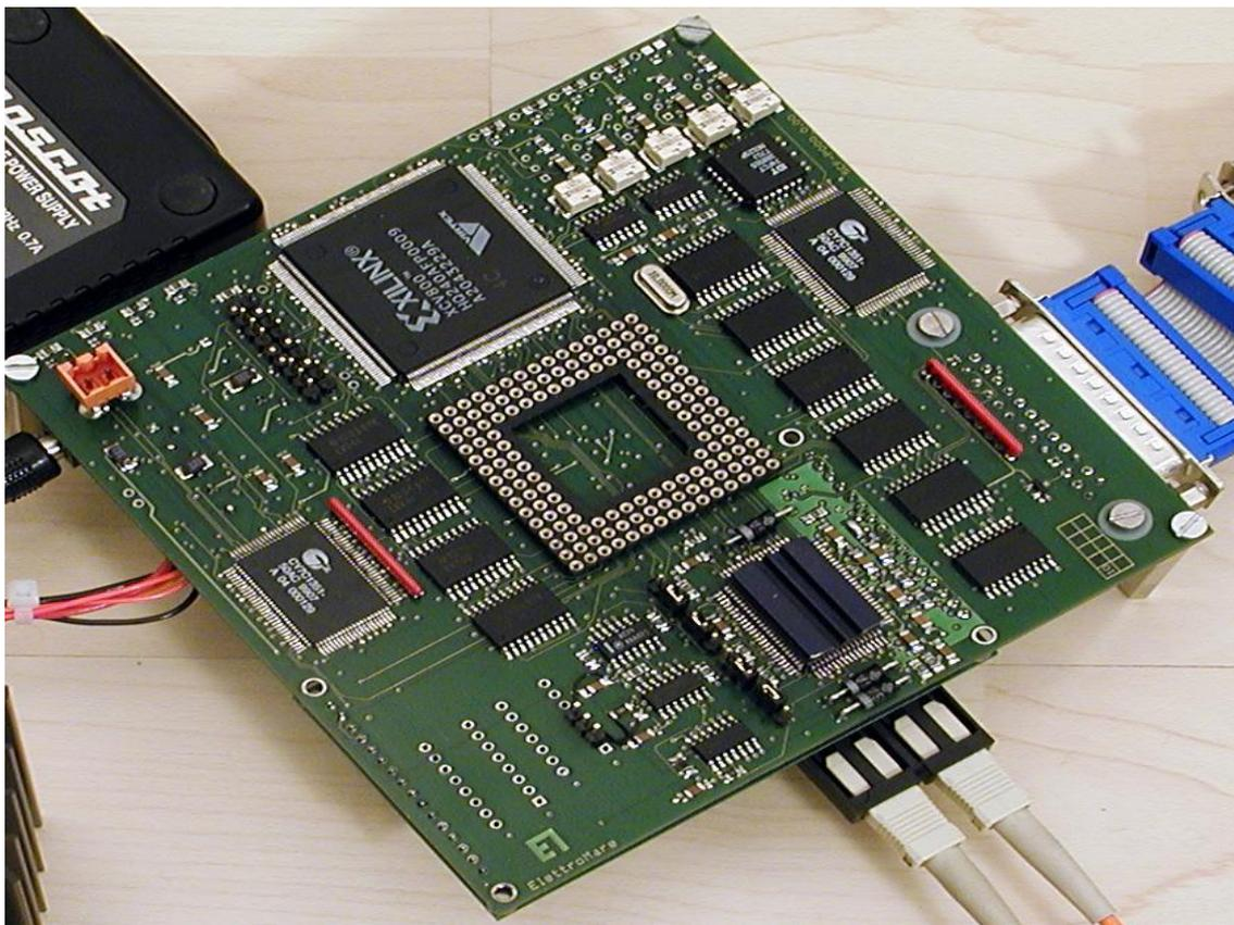
**Figure 2.** Electronics board (the APS socket is the central one).
