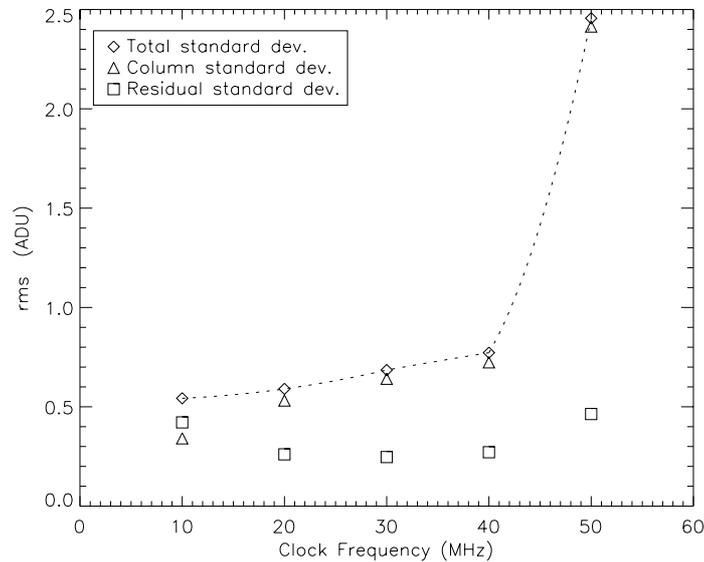
**Figure 6.** Rms noise on dark frames at different readout frequencies. The rms on raw frames is shown together with the rms after subtraction of the column FPN and the standard deviation of the column response.
