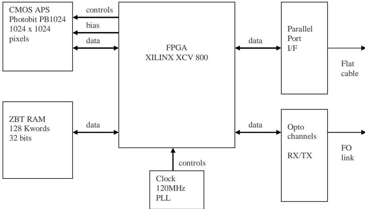
**Figure 3.** Block diagram of the PC-IAPS electronics.
