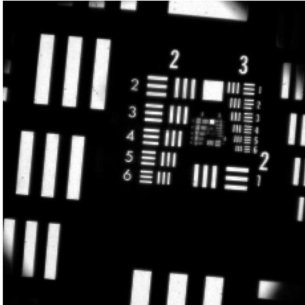
Figure 7. Image of the USAF Test Target
