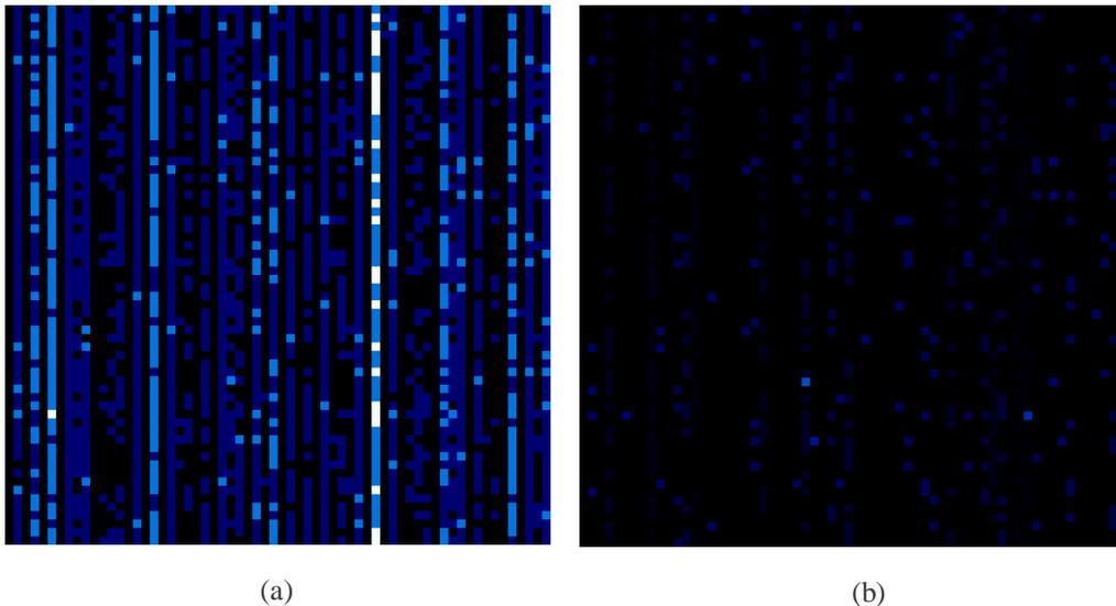
**Figure 5.** A region of a dark frame showing ‘column’ FPN (a) and a region after FPN subtraction (b)
