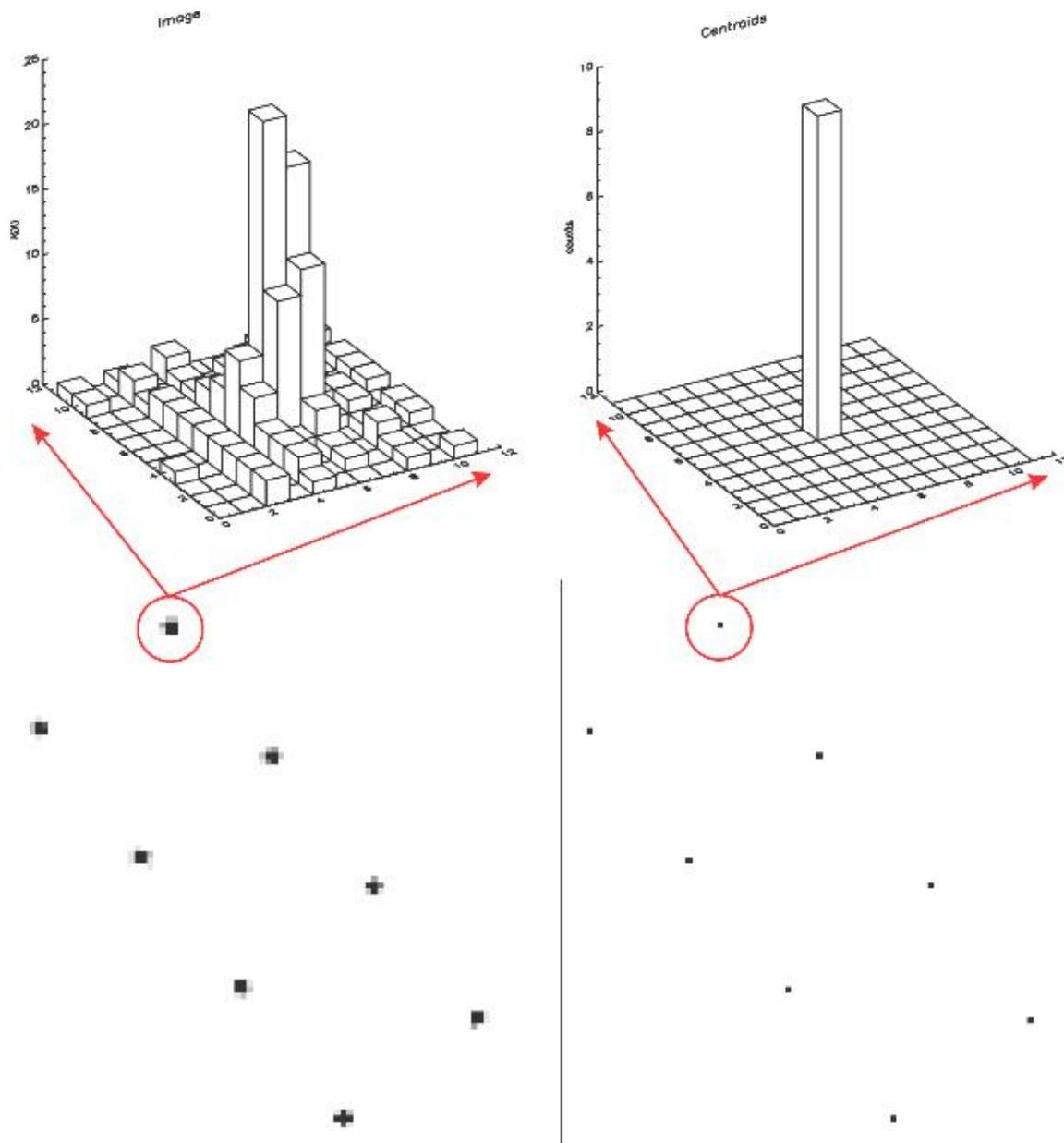
**Figure 11.** Image of a pinhole mask: (a) direct imaging, (b) reconstructed from event centroids (sampling: 1 bin/pixel).
