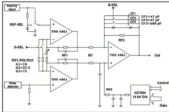
Figure 2. Preampifier (one channel)
