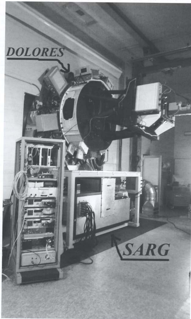
Fig. 1 - SARG layout in the TNG Nasmyth room B. On the foreground, the SARG electronic rack. Behind it, the SARG, rigidly mounted on the telescope fork. Light reaches the spectrograph from a folding mirror (in this picture hidden by the DOLORES structure). The rotator adapter is kept fixed when using SARG. Field derotation is achieved by means of an optical derotator. Guiding is done at the slit, using a cooled CCD.
