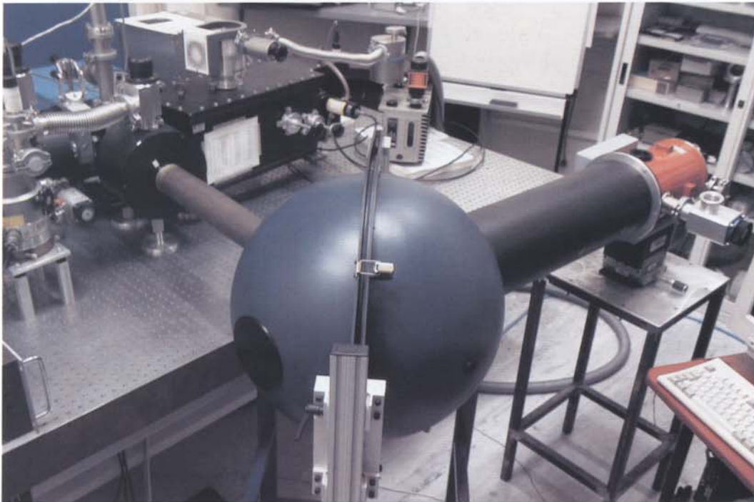
Figure 10. Set-up apparatus for linearity and uniformity measurements at Catania Observatory Detector Laboratory
