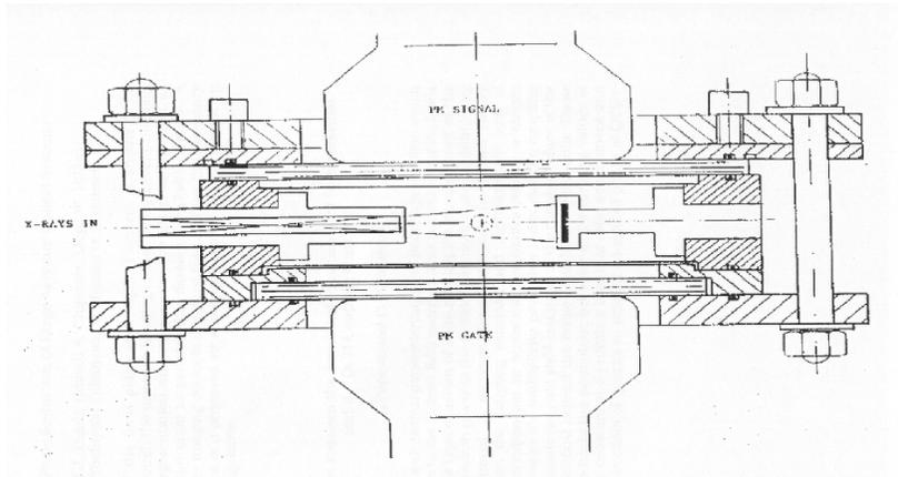
FIGURE 1. Schematic of gas cell.
